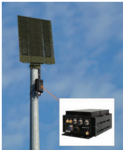
The Mercury model 6350 sensor and signal-processing system is designed to sit directly behind the antennae.
